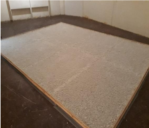
Measuring set-up in the reverberation room
